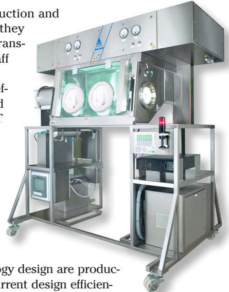
Powder handling isolator for vessel charging. Photo courtesy SKAN US, Inc.
