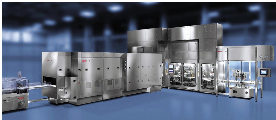
Figure 1. An isolator system showing (from left to right) a rotary washer, a sterilization tunnel, an isolator with an accumulation area, filler and stopper insertion station, and a RABS hood with a capping station. Photo courtesy of Bosch Packaging Technology.
